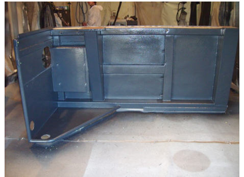
Left: Battery box sandblasted & prep Below: Battery box with Rhino Tuff Stuff
