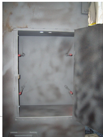
Left: Battery box sandblasted & prep Below: Battery box with Rhino Tuff Stuff
